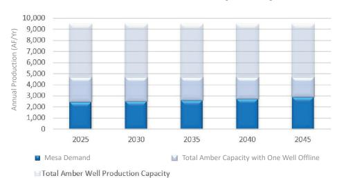
Up to 2,000 AFY can be reliably delivered from the MWRF with Well 11 offline
